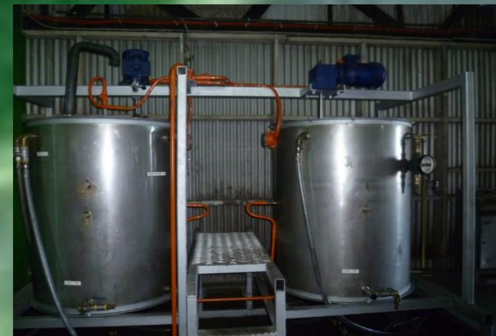
Batch processors used in the Pacific for processing coconut oil to biofuel.
